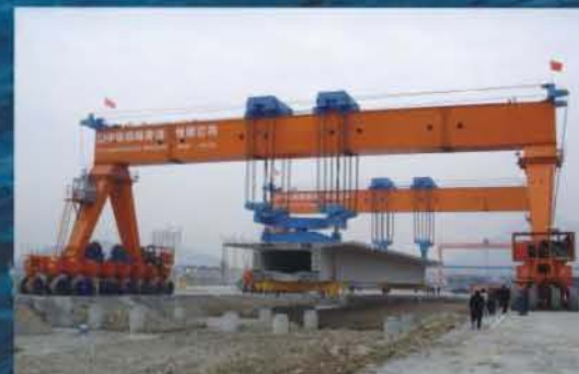
2*900T straddle carrier for China Zhoushan Bay Bridge in 2005
