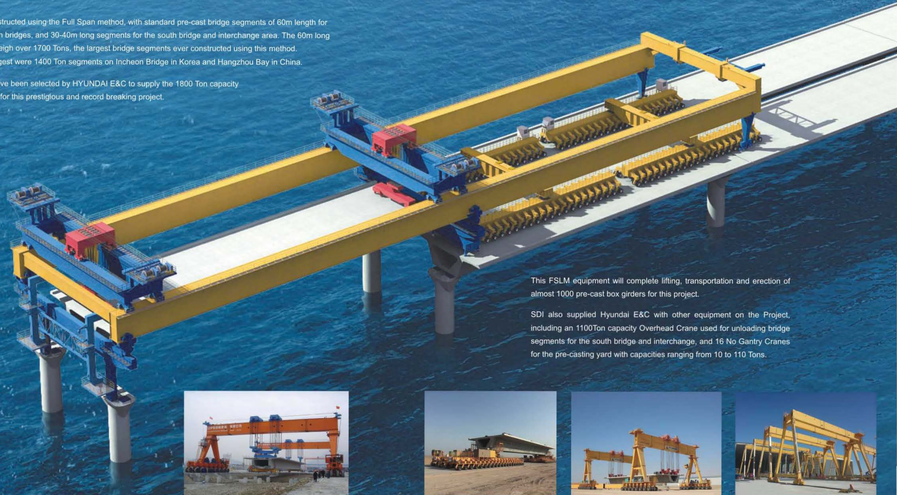
2*900T straddle carrier for China Zhoushan Bay Bridge in 2005
